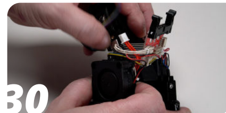
30 Attach the part cooling and heatsink fans to the SLS printed bracket using the same four M2x6 as on stock bracket.
