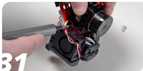
31 Two screws above the fan on each side.
