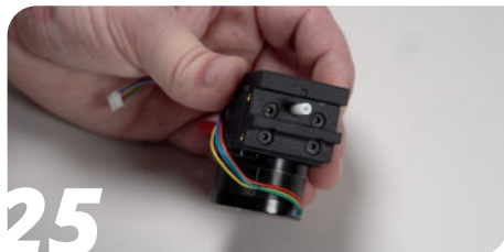
25 Insert 13mm PTFE tube.
