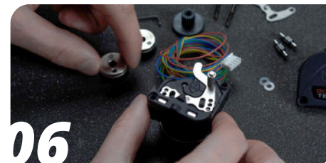
06 Remove the drivegears
