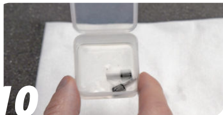
10 Put the parts in the IPA bath and leave them there for a while
