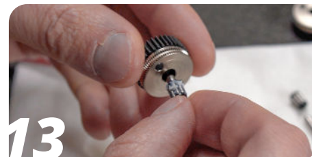
13 Place the lubricated needle bearings and pins in the drivegears
