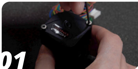
01 Undo the two M3 screws using a 2mm hex key
