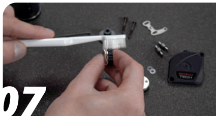
07 With a toothbrush, clean the gears
