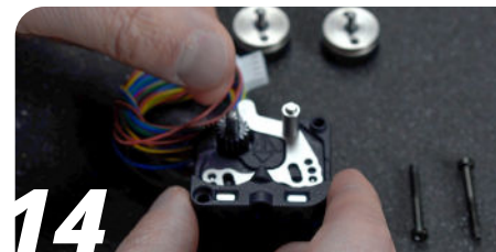
14 Insert the 4mm pin into the double gear with the rounder side facing up
