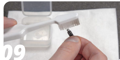
09 Dip the toothbrush in the alcohol and brush the needle bearings while on the pins
