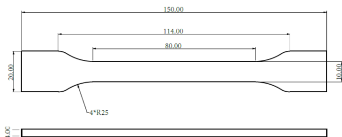
Tensile testing specimen; ASTM D638 (ISO 527, GB/T 1040)
