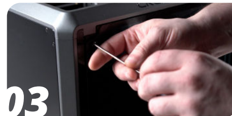
03 Remove the two front screws of the printer door using a 2mm hex key.
