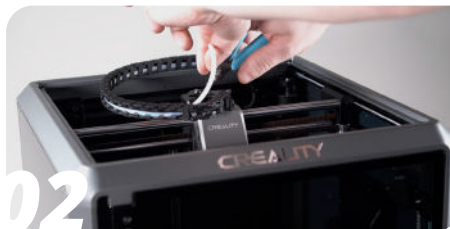
02 Cut filament a couple of centimeters above the toolhead. This can later be used as a guide for the new extruder.
