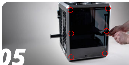
05 Unscrew and remove the enclosure panels using a 2mm hex key.
