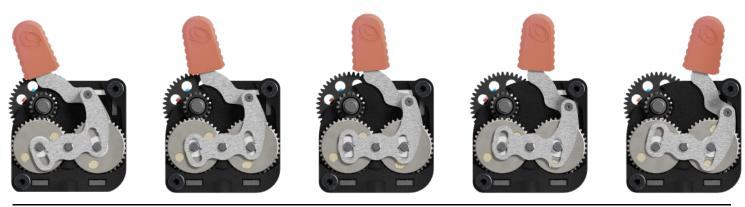
Position 0 Load or unload filament without pressure from the drivegears.
