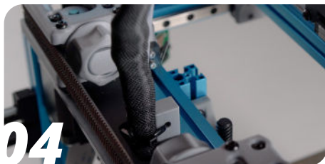
04 Cut the frame side zip tie for the wiring loom.
