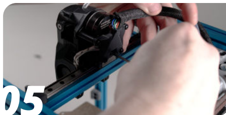
05 Undo the screws holding the toolhead in place.
