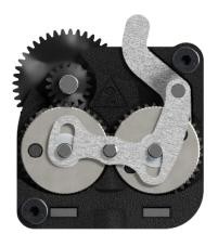
Position 0 Load or unload filament without pressure from the drivegears
