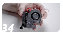
Tighten it carefully using a 2.5 mm hex key.
