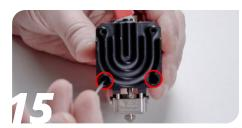
Take your LGX ACE and unscrew the two screws holding the hotend to the extruder from the front using a 2 mm hex key.
