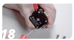
Unscrew the top right and bottom left screws on the extruder motor as seen from the back using a Philips head screwdriver.
