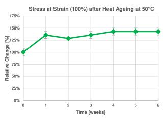
**Test parameters:** ASTM D412: Type Die C, Pull speed: 500 mm/min, 22°C
