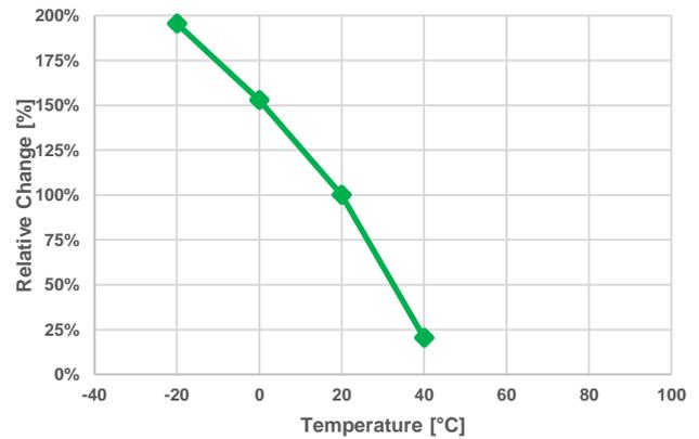
Test parameters: ASTM D638, Type IV, Pull speed: 50 mm/min, Young's modulus measured at 0.1-1% (regression),
