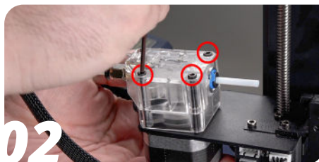
02 Remove the three M3 SHCS screws in the extruder with a 2.5mm hex key.
