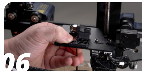
06 Fasten the bowden coupler from below using two M3x6 BHCS and a 2mm hex key. This is an optional part which can be bought in our store. Link here and here .
