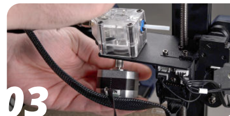
03 Remove the extruder stepper motor.
