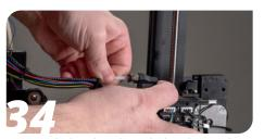
Connect the bowden tube in the bowden coupler.
