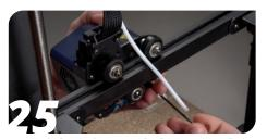
Reattach the cowling using the four M3 BHCS from before with a 2mm hex key.
