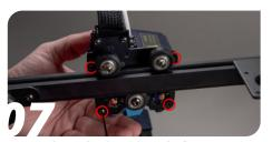
Loosen the cowling by undoing the four M3 BHCS screws in the back using a 2mm hex key.
