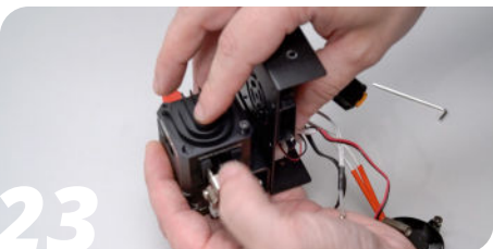
Add the hotend assembly to the extruder.
