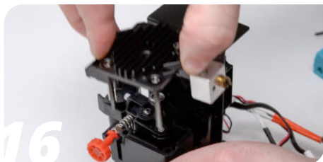
Remove the hotend heatsink.
