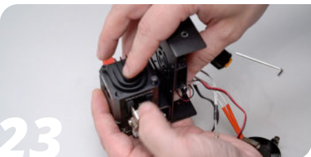
Add the hotend assembly to the extruder.
