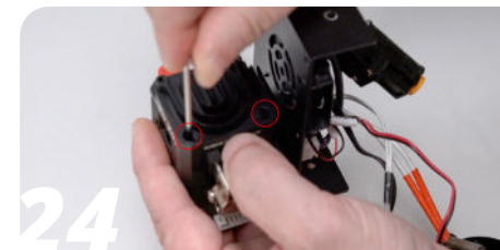
Fasten the two M3 screws at the bottom using a 2 mm hex key.
