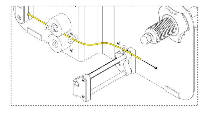
The filament must pass under the empty spool. Let it go until the diameter will remain quite constant. Then you can fix the filament to the spool.
