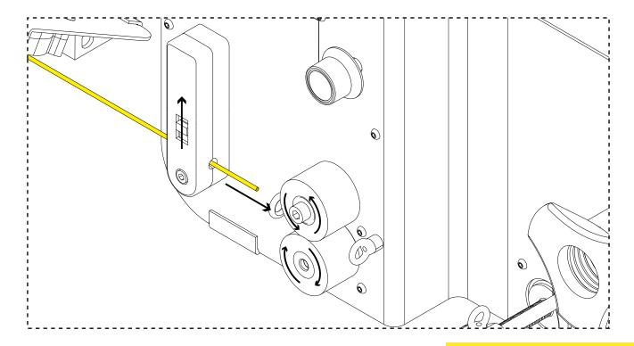
Once the filament is pushed in the measuring system the puller wheels will start to rotating and the following information will appear. This is the main working interface of Felfil Spooler.
