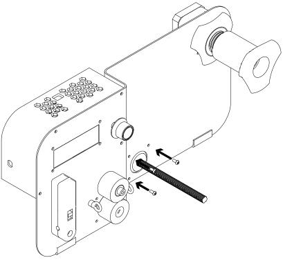
Screw the linear guide 5B into the bottom right hole.
