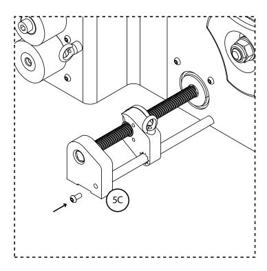
Connect the leadscrew shaft stepper to its wires connector.
