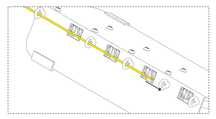
Insert the filament into the measuring system sliding up the little lever. Once the filament is in position the puller wheels will start rotating.
