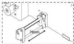
This parameter is about the spool width end. Allign the metal golfare to the spool end.
