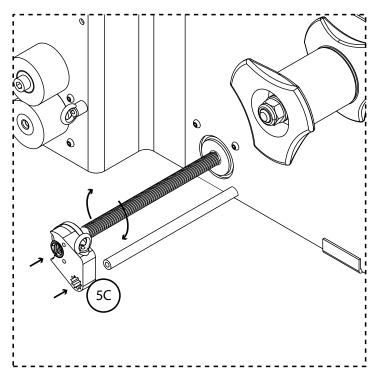
Fix the 5C component using 1 M3 screw.
