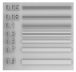
Minimum Engraved Detail Width, X-Y plane
