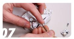
Open the extruder and remove the flow control spring.
