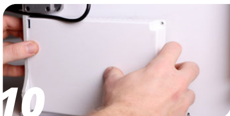
Reinstall the electronics compartment cover.
