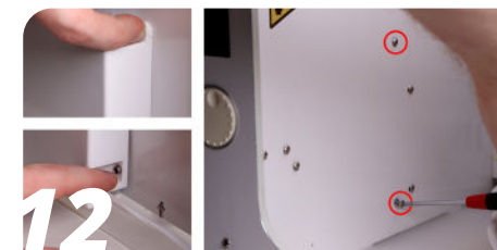
Add the two screws previously removed and tighten them back down again, holding the nylock nuts against the electronics compartment cover.
