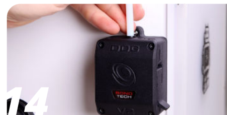
Add the bowden tube to the extruder.
