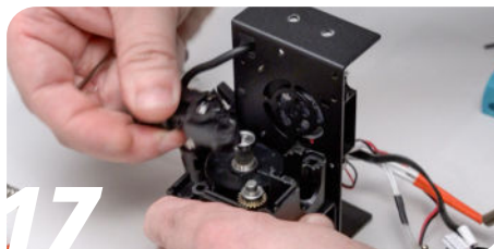
Remove the extruder tensioning assembly.
