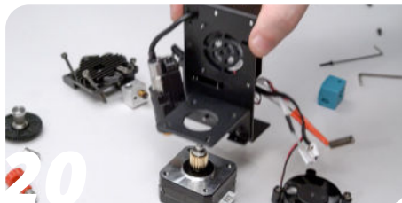
Remove the rest of the extruder and the motor from the carriage.
