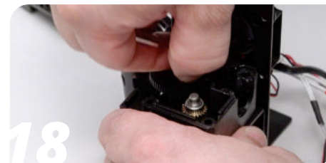
Remove the main extruder gear.
