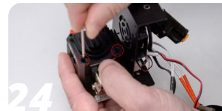
Fasten the two M3 screws at the bottom using a 2 mm hex key.
