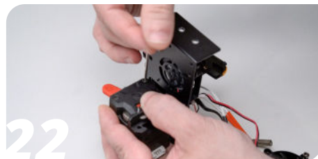
Fasten the top right M3 screw using a 2 mm hex key.
