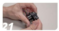
Add the mount to the bottom of the LGX lite using three low profile M3x8 screws.
