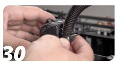
Secure the conduit to the side of the LGX lite using the two included zip ties.
