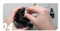
Take out the old ball bearings from the rear and front body.
