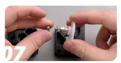
Place the other ball bearing on top of the new IDGA shaft.
