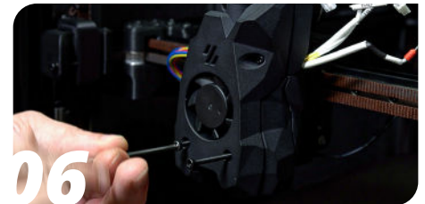
06 Add your screws for the front, make sure the upper ones are M3x16 SHCS if you're using the LGX lite
