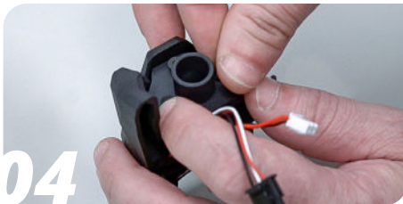
04 Place the CPAP hose mount on the top and add the four M3x6 FHCS
