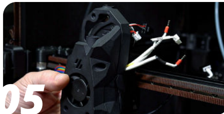
05 Pass your fan and LED wires through
