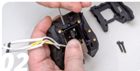
02 Insert the two M2.5x10 SHCS screws and tighten them
