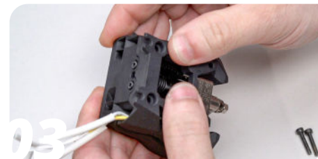
03 Place the hotend mount rear piece on the assembly
