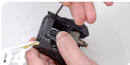
04 Add and tighten the two M3x16 SHCS screws
