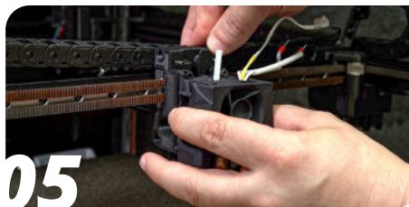
05 Add the hotend to your x-carriage, insert PTFE and connect wires according to your specific setup
